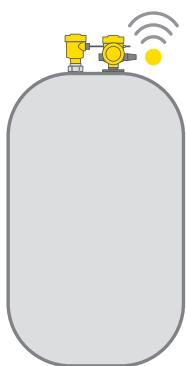
The wireless communication devices are used when measured values have to be transferred from remote monitoring stations or mobile tanks to data collection centers. They also enable wireless remote diagnostics and maintenance of the connected sensors.
