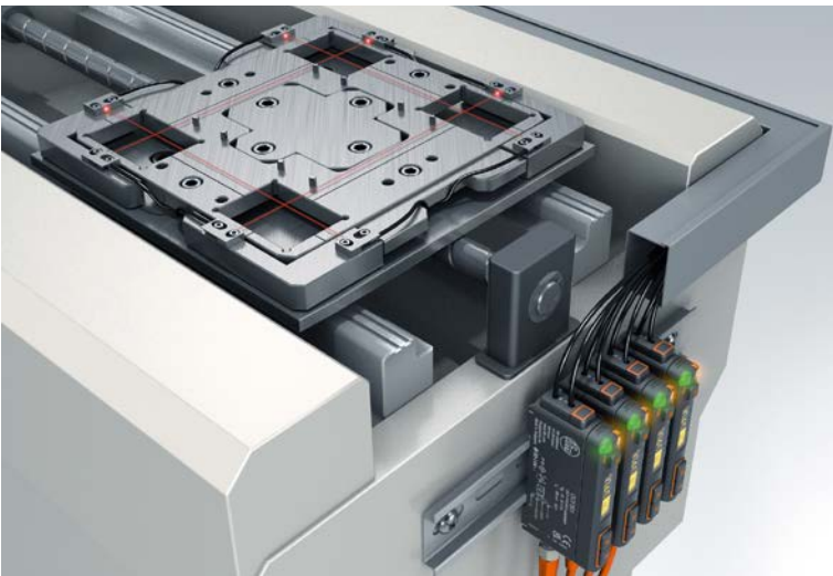
The OCF fibre optic amplifiers can be installed on a DIN rail to save space. From there, the fibre optics lead directly to the measuring points at which objects or positions are detected.
