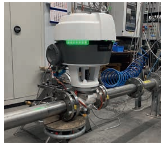
FOCUS-1 Smart meter valve for flow and decentralised process control
